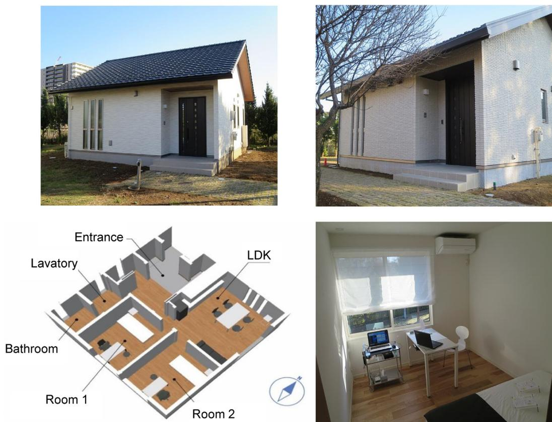
**Fig. 1.** Evaluation tests conducted in the LHs. Upper left: LH-A (typical Japanese wooden house), upper right: LH-B (light-gage steel structure), bottom left: house plan of LHs, and bottom right: an LH bedroom.
